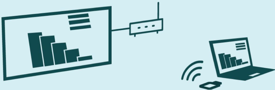
*Hardware systems use a sender that plugs into the client device with either an HDMI or USB interface.*
