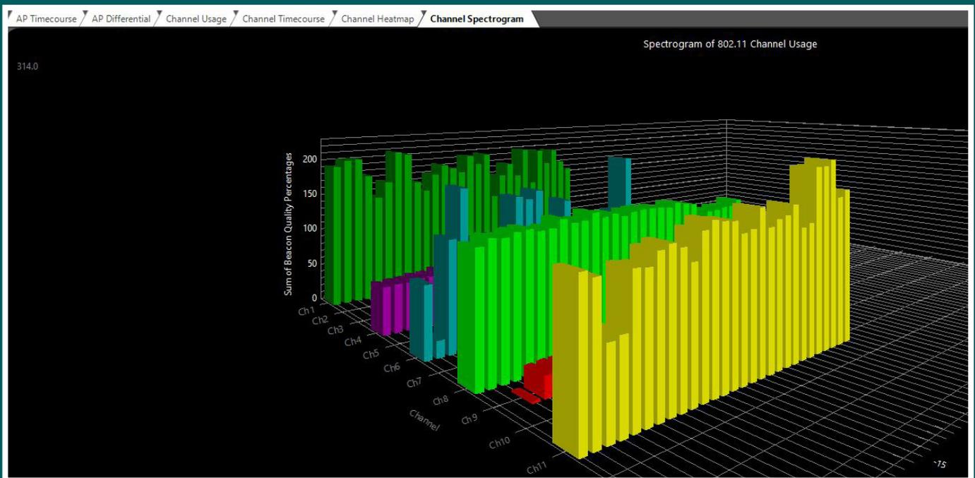
*Before deploying any wireless system, take time to do a site survey using a Wi-Fi scanner application. Avoid congested wireless channels to ensure signal stability and consistent performance.*
